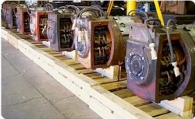
Super Lube® Silicone Dielectric and Vacuum Grease has superior vacuum capabilities for rebuilding electrical traction motors used to power passenger trains. Part of the process involves varnishing the motor components with an insulating material. The varnish must be kept from coating the commutator, bolt holes, threaded fittings, bearing shafts and electrical connections.
